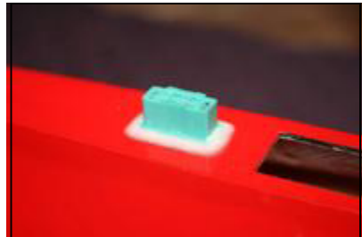
Multiplex plug epoxied into the slight recess on the fuz. . I glued a piece of balsa wood between the wing recesses inside the fuz. (access through the wing joiner hole) This was to stop the wiring loom from fowling the wing joiner when it's being inserted
