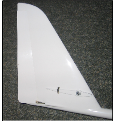
The rudder hinge is on one side like the ailerons ( Not central)
