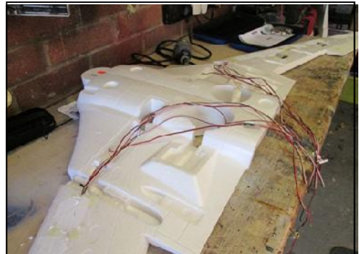
Wiring loom for lights and servos
