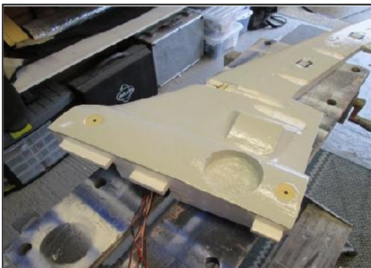
Wing now covered in Fablon ~ Note the wheel bay is partially filled
