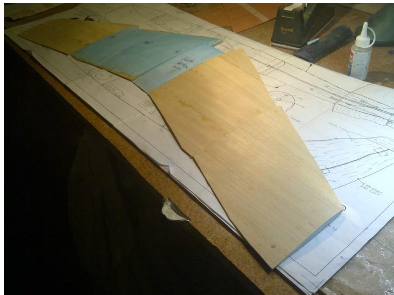
Veneer attached before trimming
