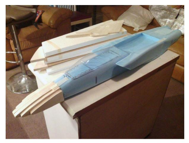
Next comes the wrapping in brown parcel tape which does not have to be smooth and is assisted with a warm solarfilm iron. The purpose of this is to firstly provide a smooth inner surface to the resin, and secondly to make the removal of the acetone laden blue foam goo from the inside.
