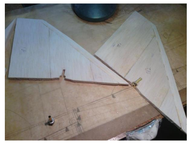
So, construction of the pivot and the position of the holes in the fuselage side has to be accurate. Some builds used a carbon rod instead of steel, which is lighter but not necessarily stronger.
