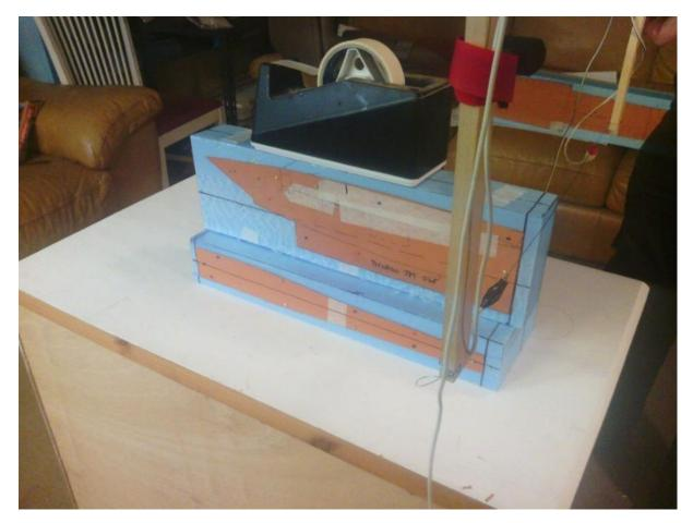
I used the same system as for wings, namely making marks at 1 inch intervals and numbering them so that both sides are cut at the same speed. I have a friend who cuts with me (Keith). It is really difficult to do it alone, but there are systems with pulleys and weights out there.
