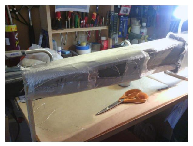
The next stage is the trickiest, mainly due to gravity. I recommend making a spit type of cradle to hold the fuselage. I use 2 lengths of wire filed to a point which are pushed into the blue foam at the nose and tail. This supports the fuselage and frees up your hands to apply the cloth. I clamp the supports to the bench.
