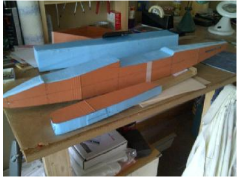
Fuselage and jet shapes with templates
