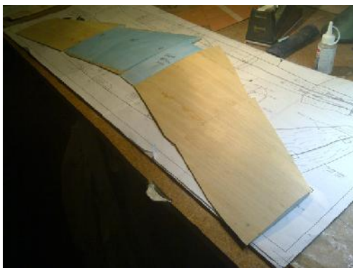
Veneer attached before trimming
