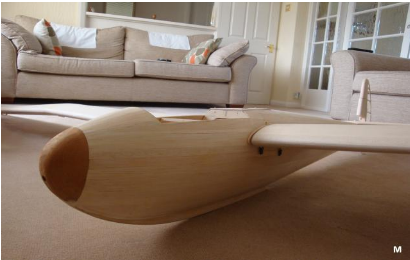
M. - The hole in the mahogany noseblock is access to the cable attachment and release mechanism. Plugged it during painting and not yet removed.
