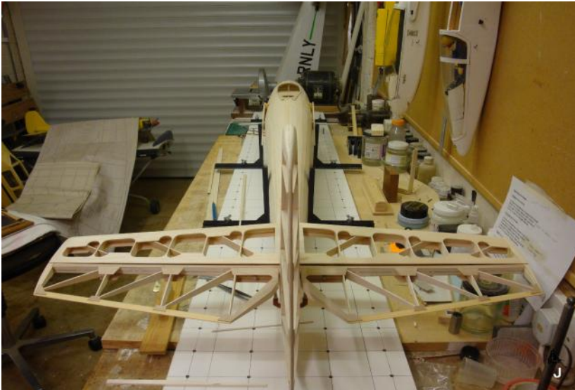
J. - Tailplane and Fin & Rudder mounted. Lots of tedious work in both.
