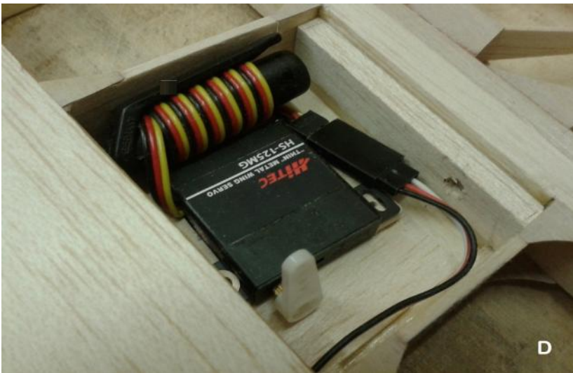
D. – How I stowed the aileron servo lead by wrapping it round a length of plastic tubing (this is actually the top of a felt pen—you can just see the clip). Double sided tape also works well..
