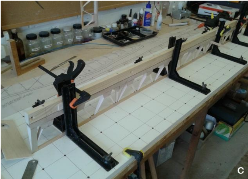
C.—Again, using fuselage jig to support aileron with hinge jig in position ready for drilling.
