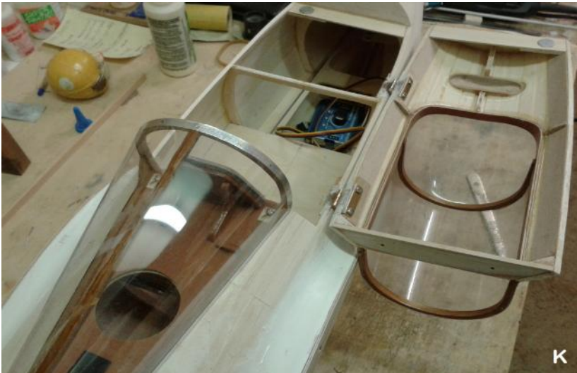
K. - Had to make special hinges for canopy because hinged edge is curved so each hinge pivot has to stand proud of fuselage edge.
