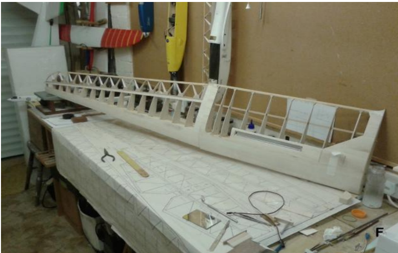
F - Wing construction complete but to facilitate handling, inner and outer panels were not joined until covering had been applied
