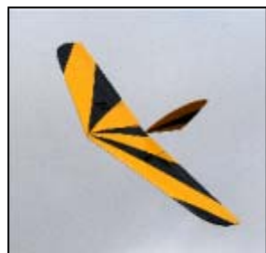
Graham Gibbons new Half Pipe in action. Wings are very sensitive to the CG position - A small change can have a profound affect on pitch control
