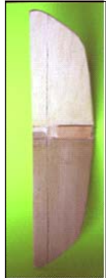
Elevator marked out on the Hatchling tail-plane
