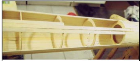
Photo 4 ~ Wing Seating to be cut out later
