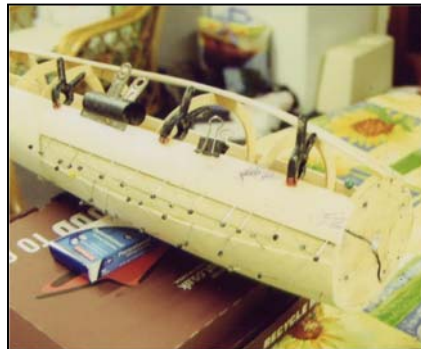
Photo 3 shows the 1/16th inch Balsa sheeting being fixed
