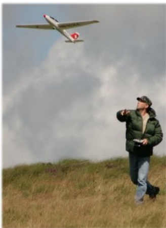
Nigel Brewer launching his 'Windrider Fox' a 66" span EPP model with rudder elevator ailerons and spoilers for landing
