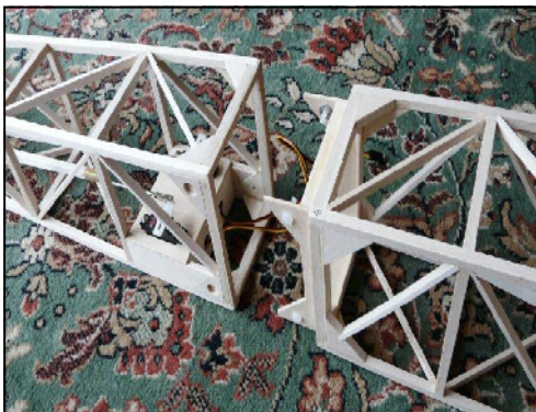
Another mod. ~ Dave's method of making the six foot long fuselage easier to transport
