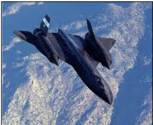
The blackbird cruised at Mach 3.2 and at that speed the outer skin would reach temperatures of around 500 deg F
